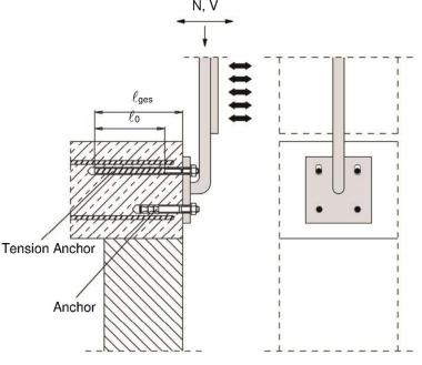
**Figure A8:** Overlap joint for the anchorage to centilever members
