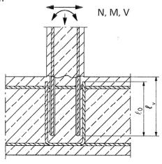
**Figure A4:** Rebar connection for components stressed primarily in compression. The rebars sre stressed in compression
