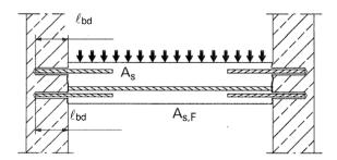
**Figure A2:** Overlapping joint at a foundation of a wall or column where the rebars are stressed in tension
