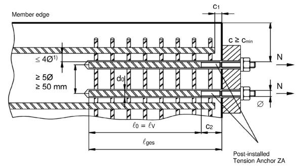
If the clear distance between lapped bars exceeds 4φ, then the lap length shall be increased by the difference between the clear bar distance and 4φ.
