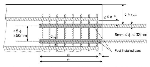
If the clear distance between lapped bars exceeds 4φ, then the lap length shall be increased by the difference between the clear bar distance and 4φ.
