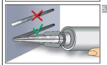
Not proper mixed mortar is not sufficient for fastening. Dispense and discard mortar until an uniform grey or red colour is shown (at least 3 full strokes).
